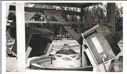
Figure 15. Implosion assembly with ionization chambers.
