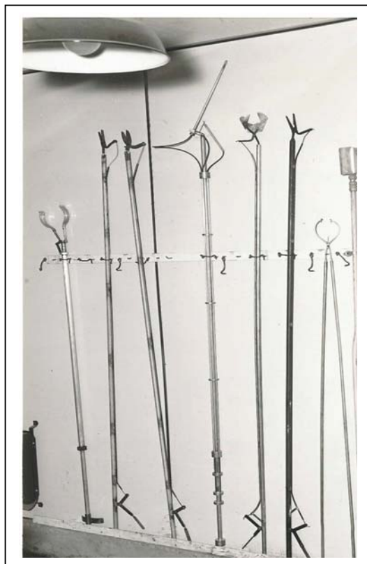
Figure 19. Remote handling tools.
